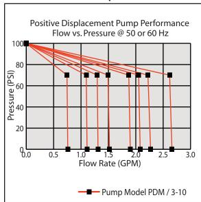
**Note:** Pump Model "PDM / 3-10" provides eight "8" selectable flow vs. pressure curves as shown. Internal valve setting shown starts coolant bypass @ 70 PSI / 4.8 bar & dead heads @ 100 PSI / 6.8 bar. Other pump curves & bypass values available upon request.
