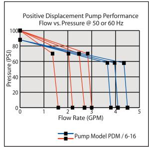
**Note:** Pump Model "PDM / 6-16" provides seven "7" selectable flow vs. pressure curves as shown. Internal valve settings shown with red lines starts coolant bypass @ 70 PSI / 4.8 bar & dead heads @ 100 PSI / 6.8 bar. Internal valve settings shown with blue lines starts coolant bypass @ 58 PSI / 4 bar & dead heads @ 88 PSI / 6 bar.
